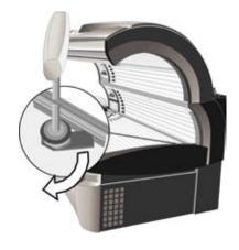
The sunbed acrylic rests in a profile groove in the front and rear side and acrros its whole length. Two sash locks secure the sunbed acrylic against unauthorized removal. The sash locks are opened with the help of an Allan key (6mm). A afety switch controls the installation and position of the sunbed acrylic.
