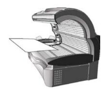
⇒ Lift the sunbed acrylic with the two sash locks pointing to the side.
