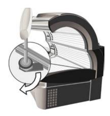
At the front and rear side, across its whole length, the sunbed acrylic sits in a profile groove. Two sash locks secure the acrylic against unauthorized opening. The sash locks are turned by an Allan key (6 mm). A safety switch controls the installation and position of the sunbed acrylic.
