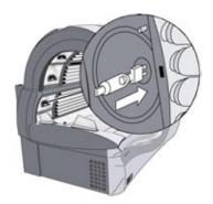
⇒ Hold the new HID lamp fast using a clean and soft, lintfree cloth and put into the lampholder.
